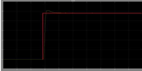
Fig. 6. PID response to rising temperature request
