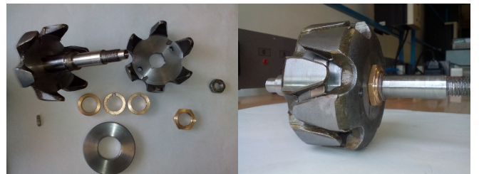
Fig. 5. The modified claw-pole rotor of the generator.
