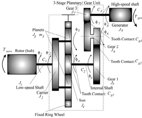
Figure 3. Dynamical model of wind turbine
