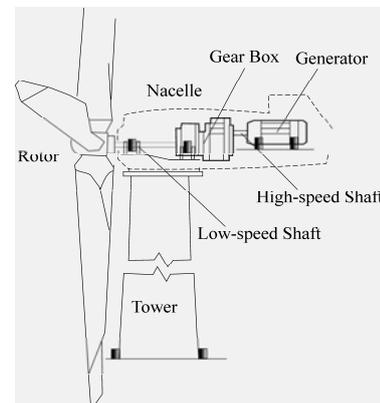
Figure 1. Schematic sketch of wind turbine
