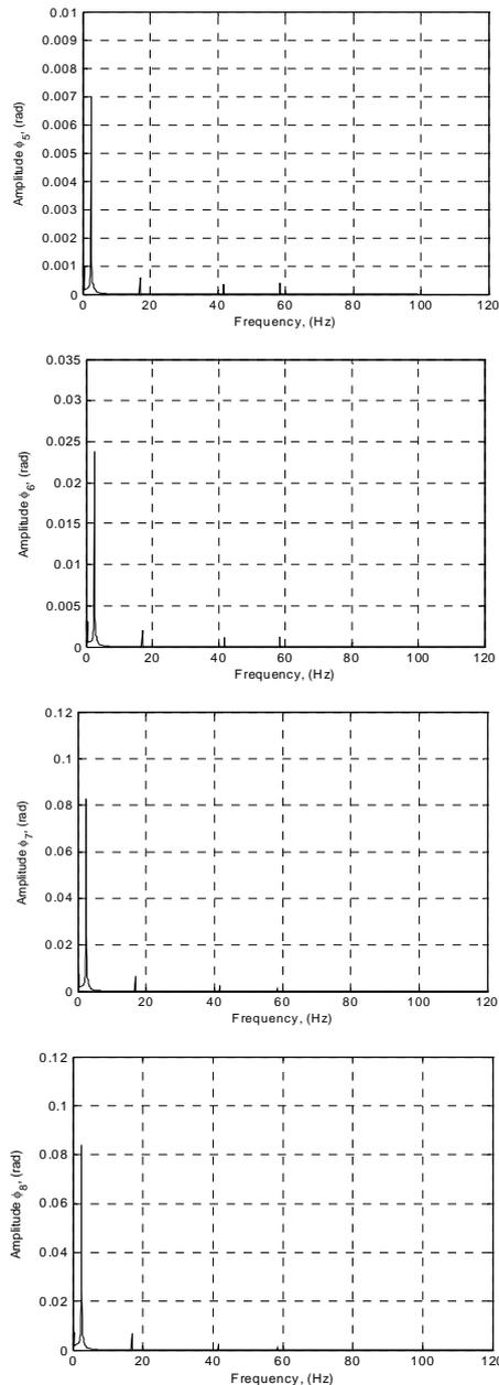
Fig. 7. Amplitude-frequency characteristics. From top: Rotor (hub), carrier, planets, sun, gear 1, gear 2, gear 3, generator rotor
