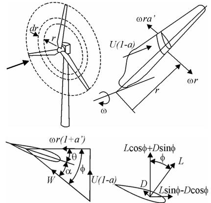
Figure 4. Blade element velocities and forces [9]
