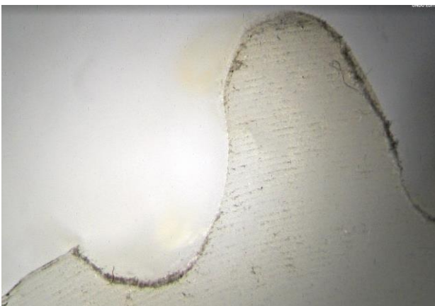
Fig. 7. Fracture and wear on cycloid gear wheel.
