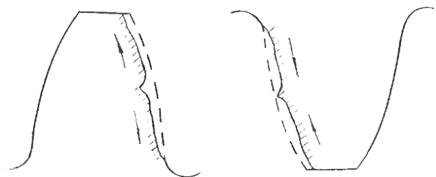
Fig. 10. Wear profiles on plastic gear flanks for (a) the driver and (b) the driven gears.
