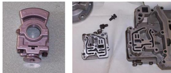
Figure 1.3. Centrifugal governor and position transmitter
