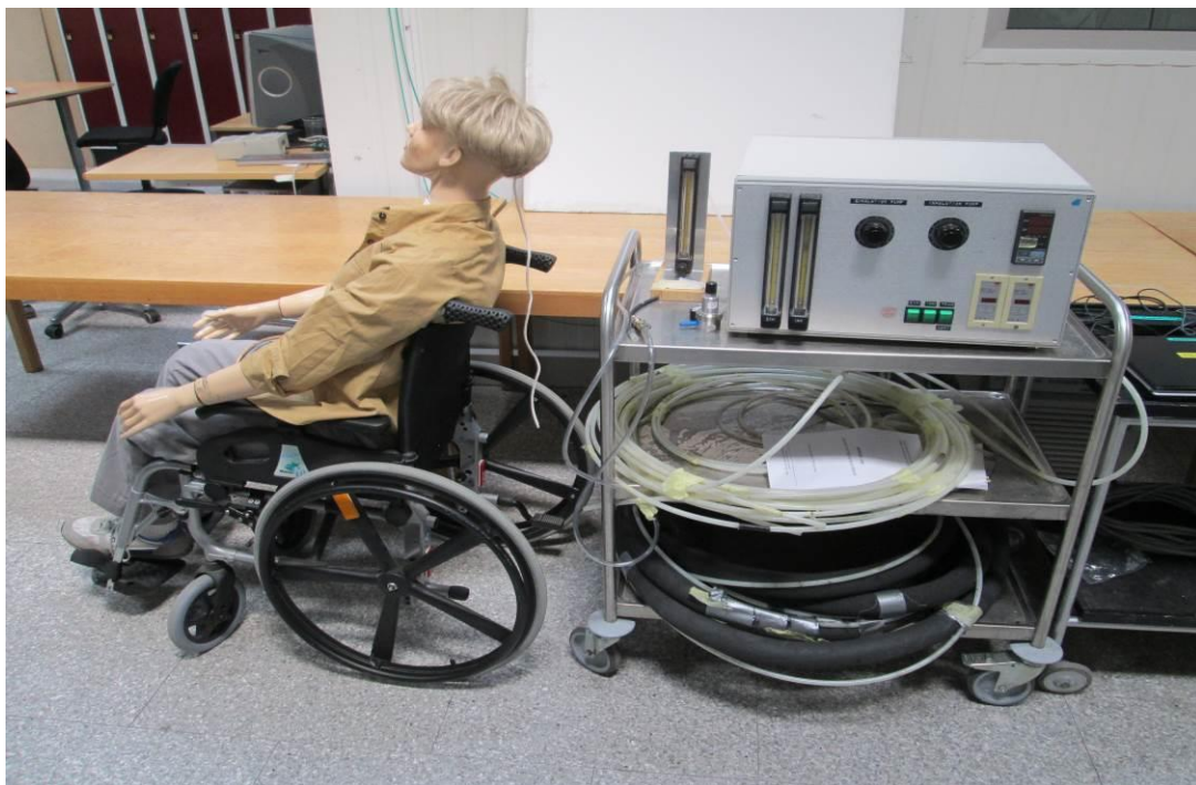
Figure 1. Breathing thermal manikin, owned by ICIEE at Denmark Technical University
