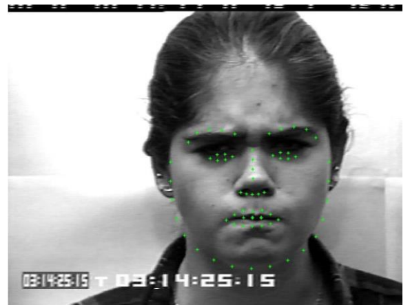
Fig.3. Anger emotion confused with disgust where eyes' feature points are incorrectly detected
