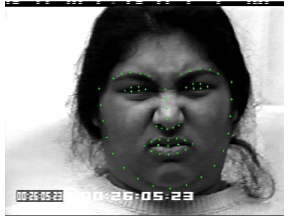
Fig.2. Disgust emotion confused with anger while all feature points are detected correctly
