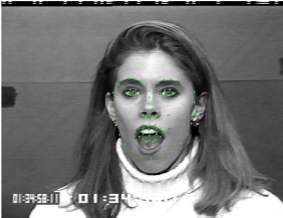
Fig.4. Surprise emotion confused with fear where lips' and partially face contour around the chin feature points are detected incorrectly
