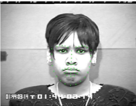
Fig.5. Sadness emotion confused with fear where lips' feature points occlude an area higher than the mouth and right part of the face contour is slightly translated to left
