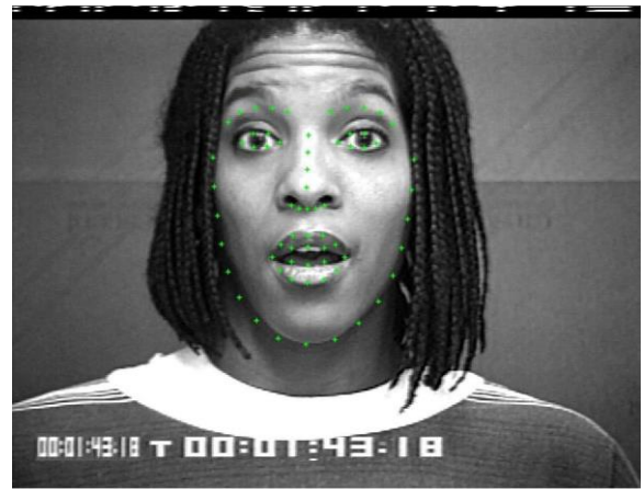
Fig.6. Surprise emotion confused with sadness where eyebrows' feature points fall below the upper boundaries of the eyebrows themselves. Left part of the face contour is slightly displaced to left
