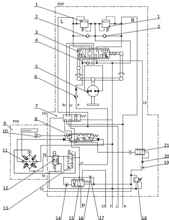
Figure 3. Hydraulic schematics of EHSU OSPE 200.
