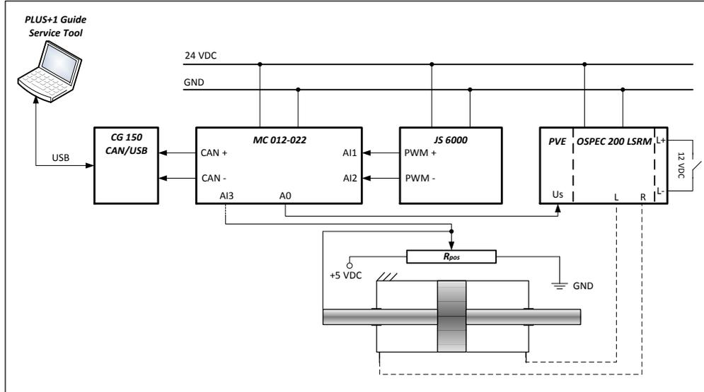
Figure 4. Conceptual representation of electrical connections of the control system
