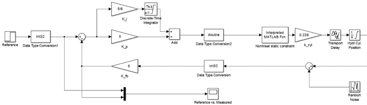
**Figure 6. Simulink model of the closed-loop digital control system**
