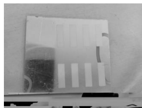
Fig.1 2 \mu\text{m} PVDF layer on PET substrate with Al top and bottom electrodes [4]
