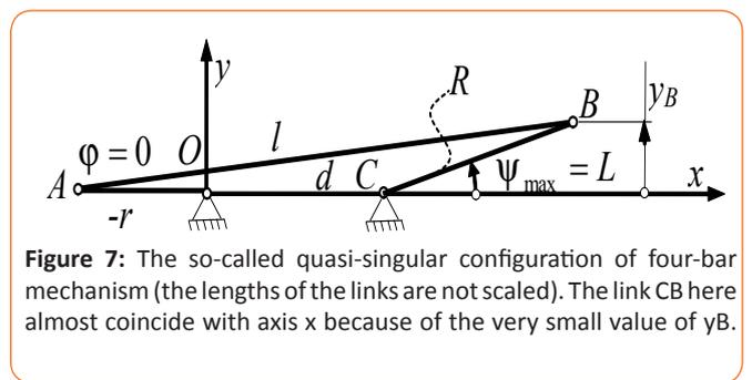
The next reason that concerns the non-linear transformation of the Freudenstein-Chebyshev method results from the quasi-singular configuration of the mechanism for  $\varphi=0$ . It follows from formula (11) and the symmetry, that the one of maximum errors has to be in the centre of the interval  $-90^\circ \leq \varphi < 90^\circ$ . Because of the very small relative error for this position, the mechanism is very close to its singular configuration, which is determined by
