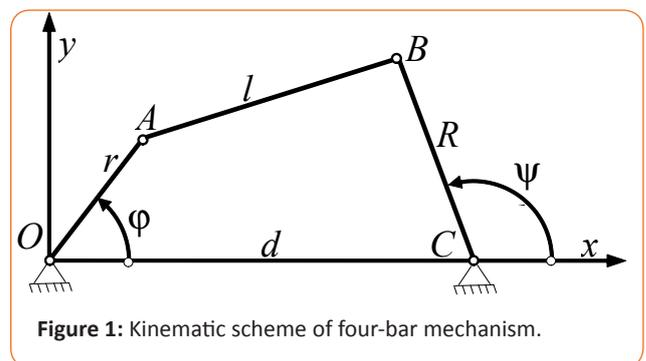
Figure 1: Kinematic scheme of four-bar mechanism.
