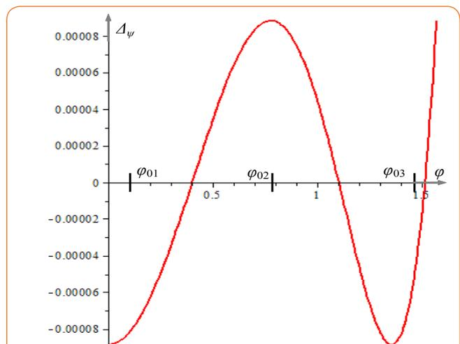
Figure 4: The polynomial of Chebyshev for  $0 \leq \varphi \leq 90^\circ$ . The precision points  $\varphi_{01}$ ,  $\varphi_{02}$  and  $\varphi_{03}$  do not coincide with the roots of the polynomial.
