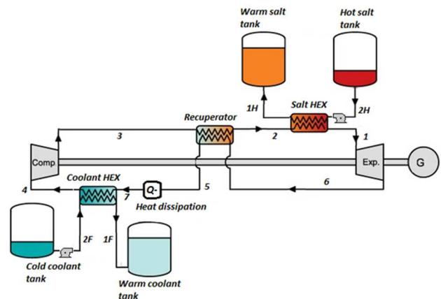
Fig. 2. Principal diagram of the discharging cycle
