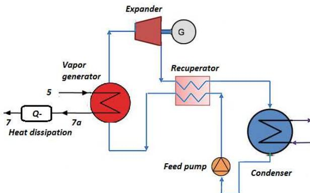
Fig. 3. Principal diagram of an ORC
