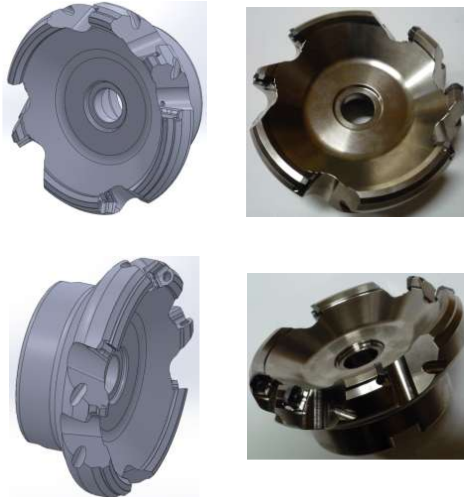
a) 3D drawing of a mill with irregular teeth pitch b) produced mill with irregular teeth pitch
