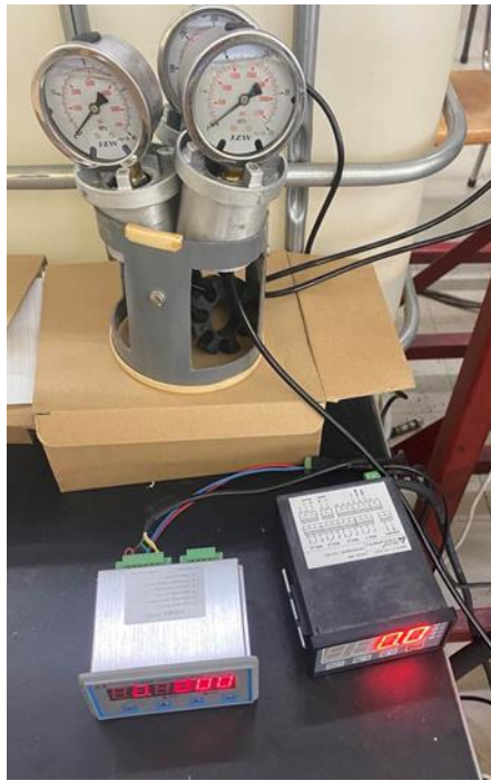
Fig. 4 Indication the hydraulic motor test, such as pressure, flow and torque.
