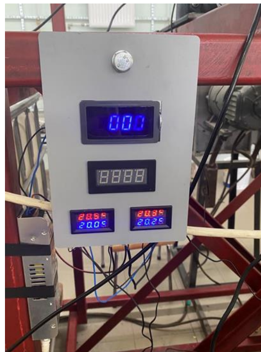
Fig. 3 Indication of revolutions and temperature of the hydraulic test bench.
