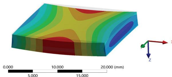
Figure 5. Deformation under uniaxial loading of the experimental body.
