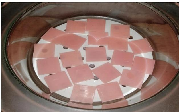
**Figure 2.** Drying of the test specimens into the desiccator.
