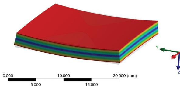
**Figure 8.** Stress when loading the experimental body - bending moment.
