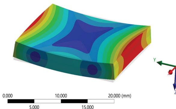
Figure 4. Deformation under load – bending moment.
