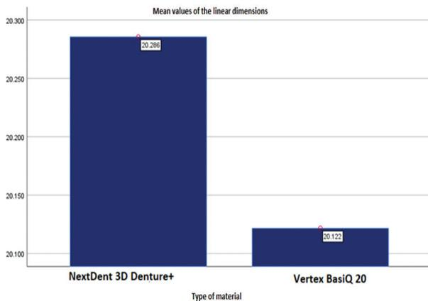
**Figure 6.** Average values for deformation (in mm) for the type of material.
