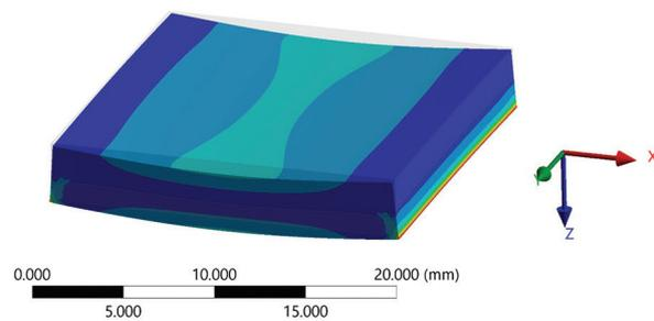
**Figure 7.** Stress during uniaxial loading of the experimental body.
