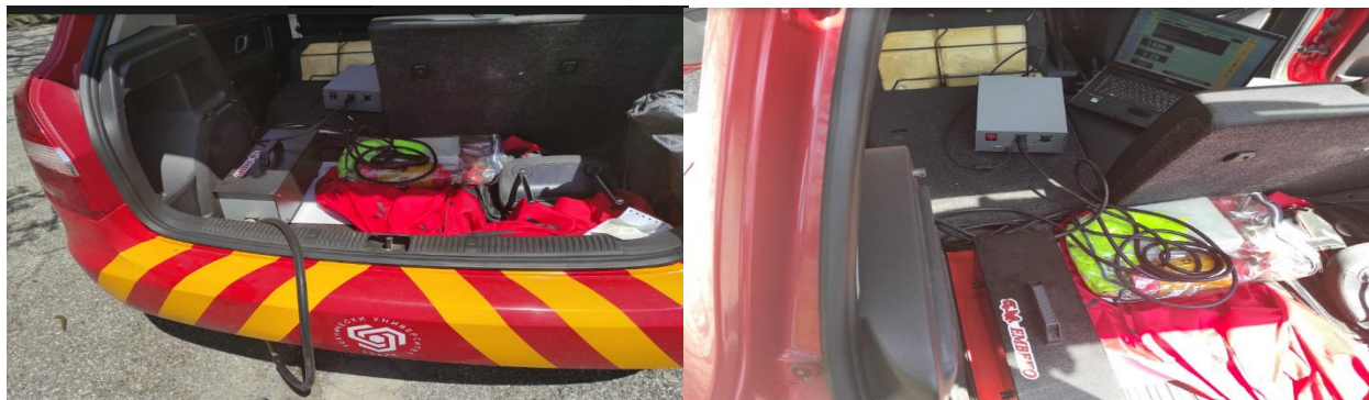
FIGURE 7. Skoda Fabia equipped with opacimeter BrainBee OPA-100 for measuring the emissions
