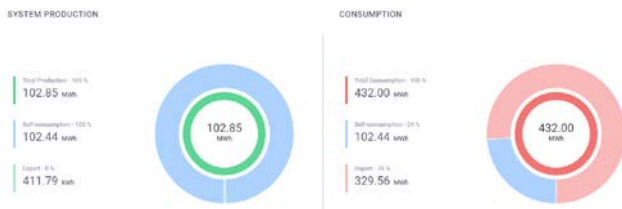
Fig. 10. Photovoltaic production and energy consumption in graphical form.
