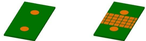
Figure 8 3D model of two antenna elements in H-plane configuration with and without implemented EBG structure between them
