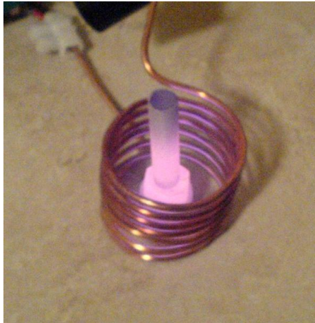
Fig.11. Photo of the heated steel detail when the surface temperature reaches 700° C.
