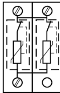
Fig. 4 Cathode arrester with varistor
