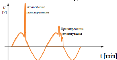
Fig.1 Atmospheric and commutation voltage peaks
