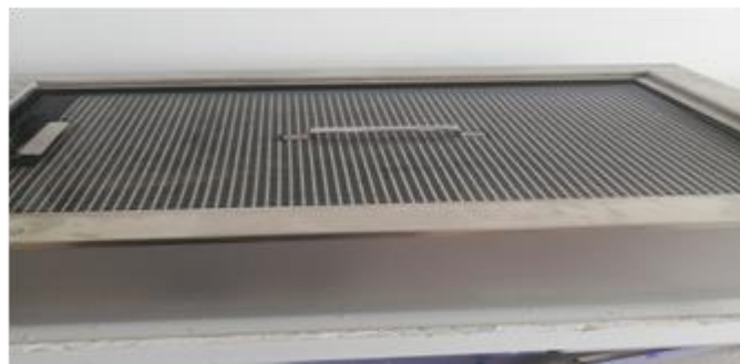
Fig. 4 The vent of the dryer
