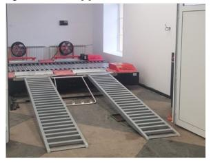
Fig. 1. Chassis dynamometer DynoCosber 4000 [6].
