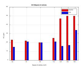
Fig. 9. Experimental study of the content of CH, [ppm] in the exhaust gases of a car Honda Civic Aerodeck 1.5 iLS.
