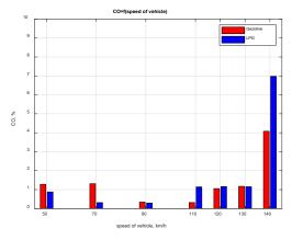
Fig. 7. Experimental study of the content of CO, [%] in the exhaust gases of a car Honda Civic Aerodeck 1.5 iLS.
