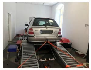
Fig. 5. Measurement of the content of toxic components in the exhaust gases.
