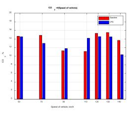
Fig. 8. Experimental study of the content of CO<sub>2</sub>, [%] in the exhaust gases of a car Honda Civic Aerodeck 1.5 iLS.
