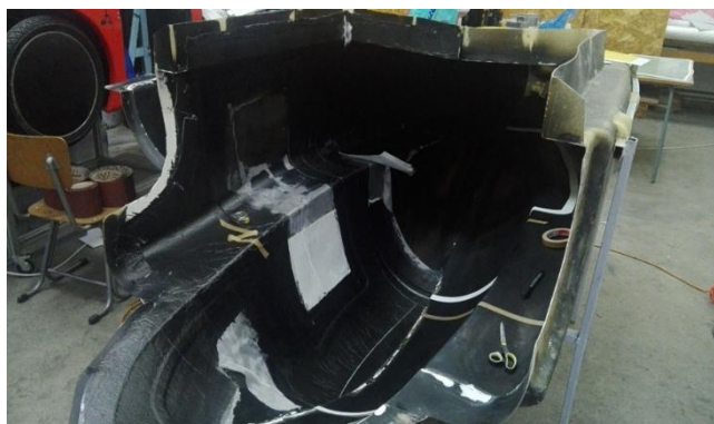
Figure 10. Cleaning and preparing the mould for hand lay-up.
