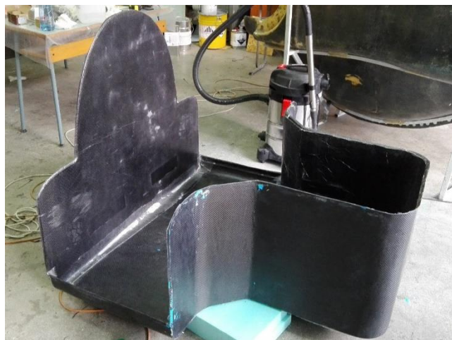
Figure 14. Separated from the mould and cleaned floor and walls.
