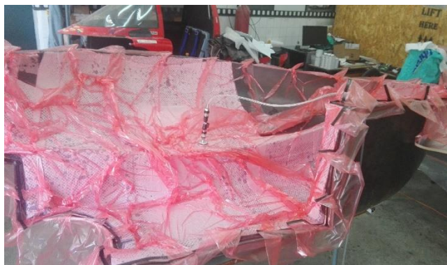
Figure 11. Vacuum bagging of the laminated moulds.
