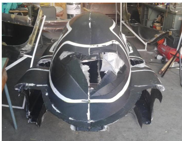
Figure 12. Carbon-fibre coupe separated from the mould before treatment.
