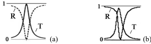
Fig. 6. The computed transmission T and reflection R around the IWS spatial resonance according to the approximate theory (a) and the exact theory (b). He-Ne laser beam ( \lambda = 0.6328 \mu\text{m} ) [1]. The parameters: \theta = 5^\circ , \alpha = 5 \times 10^{-5} rad, IWS \theta = 5^\circ , \alpha = 5 \times 10^{-5} rad.
