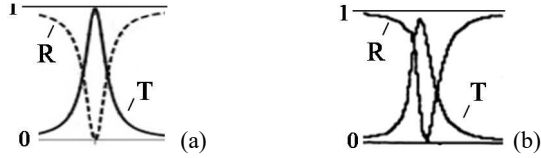
Fig. 3. The computed transmission T and reflection R around the IWS spatial resonance according to the approximate theory (a) and the exact theory (b). He-Ne laser beam ( \lambda = 632.8 nm) [1,3].
