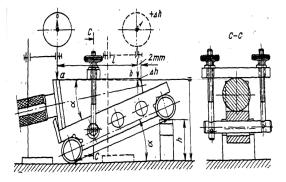
Fig. 3 principal measurement of a taper angle of outer cone with sine bar [3].
