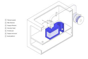
Fig 5. Schematic diagram of FDM technology.
