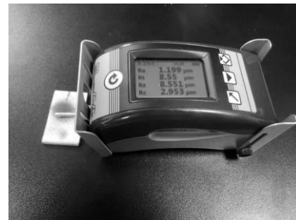
Fig. 2. Measuring of the microhardness after wear Fig. 3. Measuring of the roughness after wear
