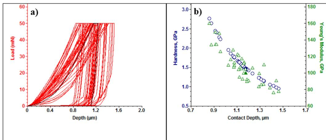
Fig. 5. a) - Nanoindentation curves; b) - hardness (H) and elastic modulus of light-activated coatings.
