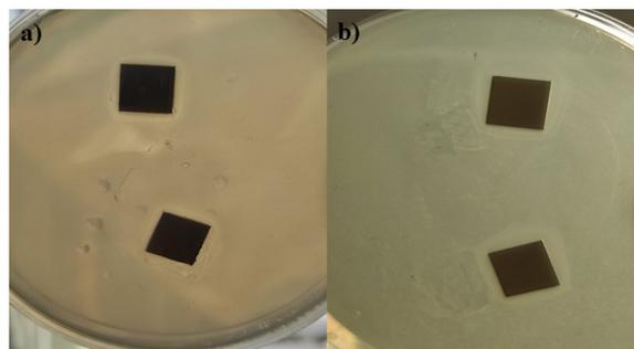
Fig. 6. Antibacterial activity of photoactive antibacterial coatings against: a) - *B. subtilis* and b) - *E. coli*.
