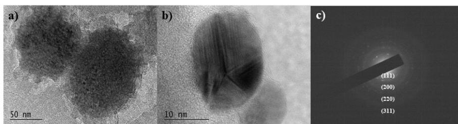
Fig. 3. a-b) - TEM analysis of PPIX-ED/AgNPs complex; c) - SAED of PPIX-ED/AgNPs complex.
