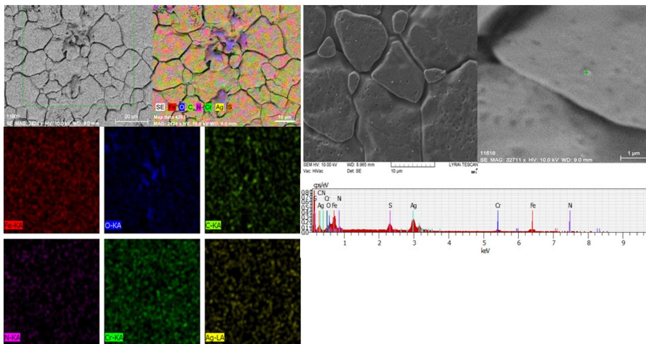
Fig. 4. EDX-SEM analysis of P(mDOPA)-co-P(DMAEMA<sup>+</sup>)/Pox(mDOPA)/PAH/PPIX-ED/AgNPs coating on SS substrate.
