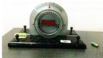
Fig. 4. Device for measuring coefficient of sliding friction
