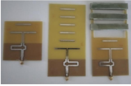
Fig. 6. The made Quasi yagi antennas
