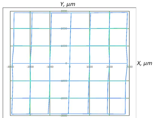
Fig. 6 Deformation of the matrix due to the non-linearity and non-uniformity of the PSD
