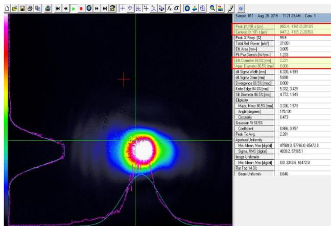
Fig. 8 Energy distribution in the cross-section of the laser beam at a distance  $L= 1400$  mm from the exit aperture of the laser beam
