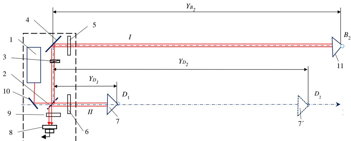
Fig. 1 Dual-channel laser system for control of surfaces mutual arrangement
