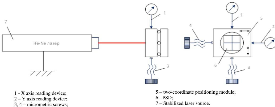
Fig. 2 Principle scheme of the setup for studying the positional characteristic of the PSD and the photoreceiving module
