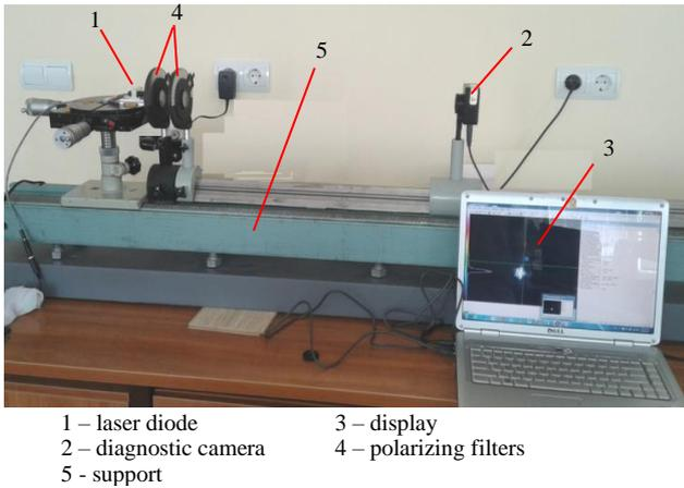
Fig. 7 Experimental setup for studying the structure of the laser beam
