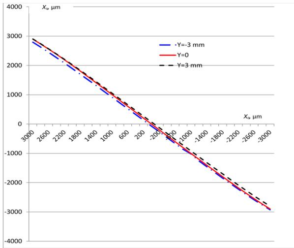
Fig. 4 Direction characteristic of the PSD
