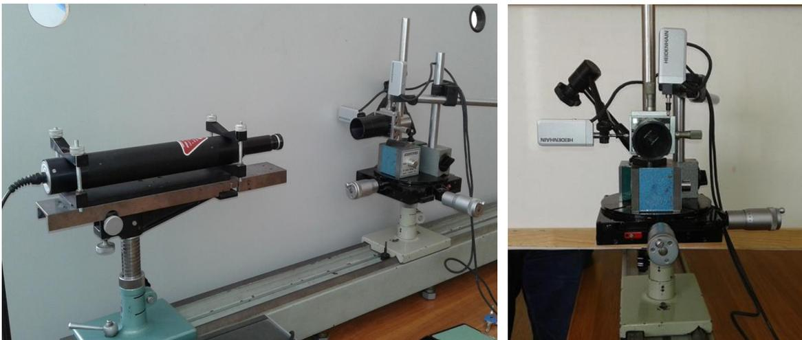
Fig. 3 Experimental set-up for studying the characteristics of PSD
