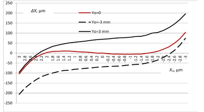
Fig. 5 Measurement error  $\Delta X, \mu\text{m}$  of the X coordinate of the center of the laser spot
