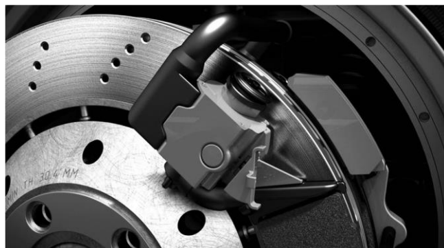
Figure 5: Prototype of a vacuum cleaner installed on the brake disc for collection of PM.
