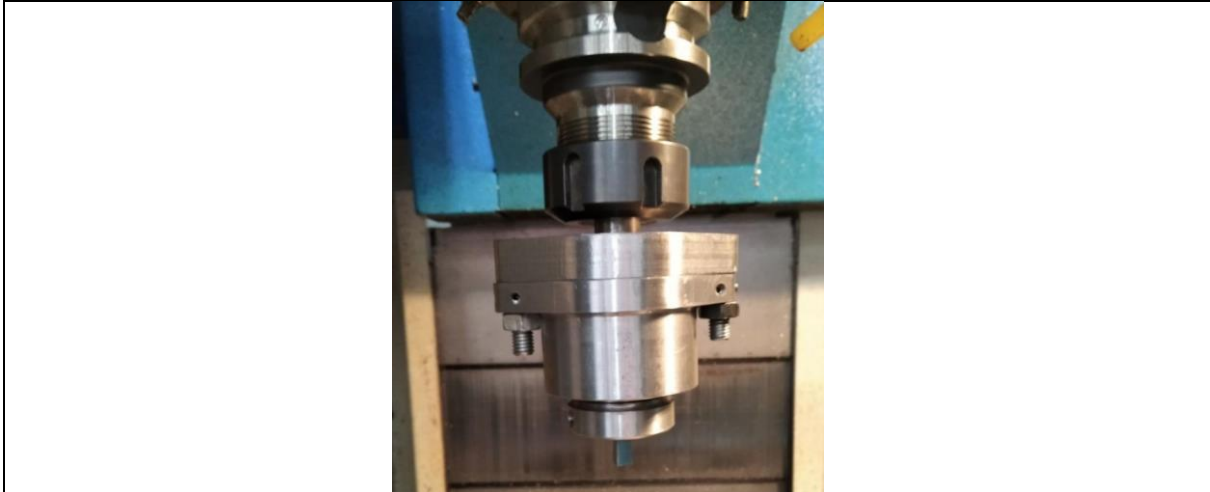
Figure 12: Adjustable toolholder installed in the spindle of the machine
