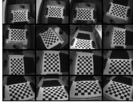
**Fig. 13.** The sequence of images of the test pattern used for geometric camera calibration
