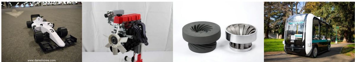
fig. 7. Example of 3D printed objects: a) – FDM RC F1 racing car [13]; b) FDM and SLA-printed scaled replica of an internal combustion engine [15]; c) sand mold made by binder jetting and the metal object created by sand casting using the same mold; the same metal part can also be produced by using SLS or LMD [23]; d) autonomous electric shuttle “Olli” with 80% of the parts and components being 3D printed [20].
