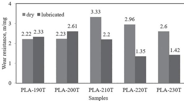
Fig. 7. Wear resistance at L = 37.65 m
