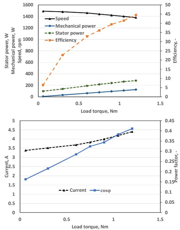
Fig. 6. Measured operational characteristics of the laboratory used single-phase induction motor.
