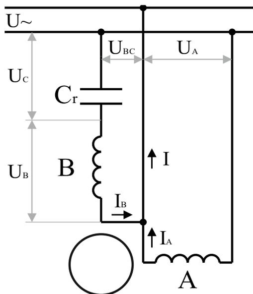
Fig. 1. Schematics, describing the operating principle of a two-phased induction motor with a single-phase power supply and a run-capacitor
