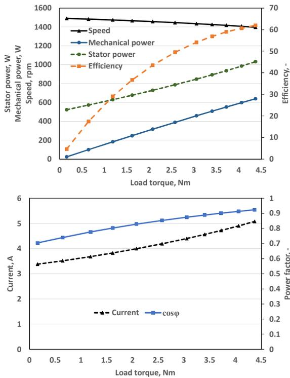
Fig. 5. Operational characteristics of the modelled single-phase induction motor.
