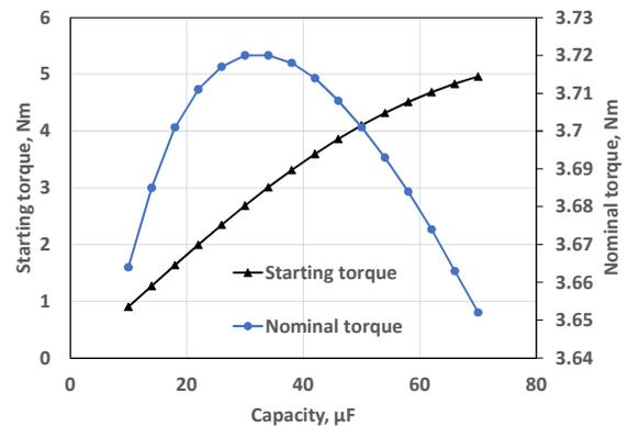
Fig. 4. Starting and nominal torque in dependence of the chosen capacity of the run-capacitor used in the modelled single-phase induction motor.
