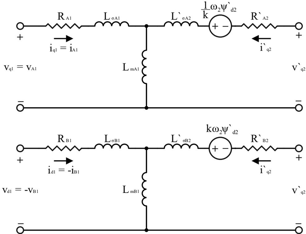
Fig. 2. Equivalent electrical circuits of phase winding A (top) and B (bottom).
