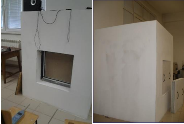
Fig.2. View of the experimental set-up used for the comparative measurements of sound insulation of materials
