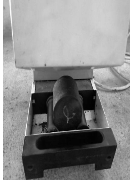
Fig. 7 Apparatus for determining friability
