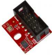
Fig. 1. The module with two sensors – BME280 (on the left) and CCS811 (on the bottom)
