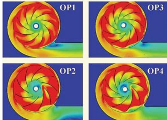
**FIGURE 12.** Visualization of the velocity distribution in OP1 to OP4.
