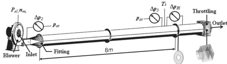
FIGURE 3. Schematic of the air-measuring test section with integrated S-HP 470/35-105/20 radial high-pressure air blowers.
