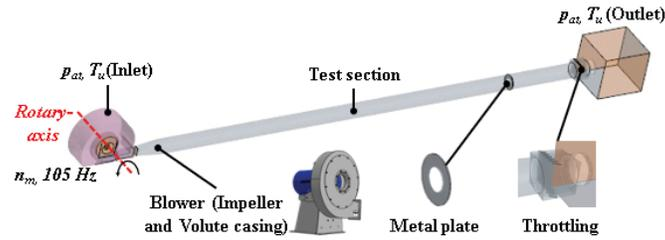
FIGURE 6. 3D Numerical modeling and boundary conditions of the digital twin.
