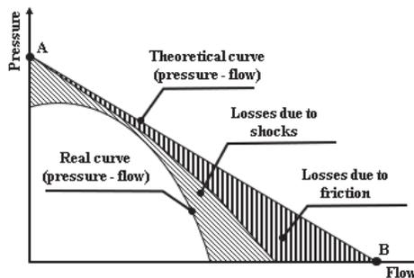
FIGURE 2. Empirical prediction of the ventilation characteristic curve [7].
