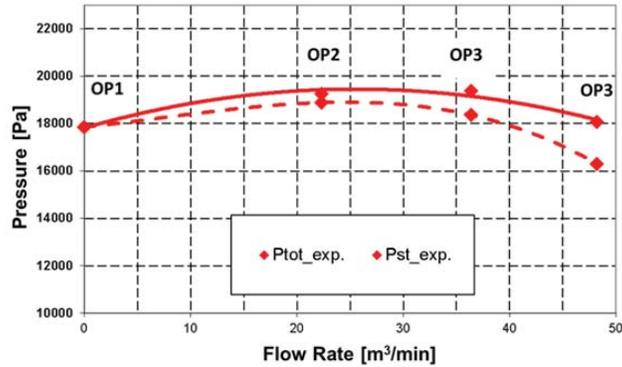
FIGURE 5. Ventilation characteristic curves of S-HP 470/35-105/20.
