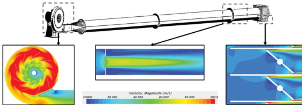
FIGURE 11. Speed distribution in the Virtual air-measuring section.
