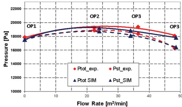
FIGURE 10. Experimental and simulated ventilation characteristic curves (static and total pressure).
