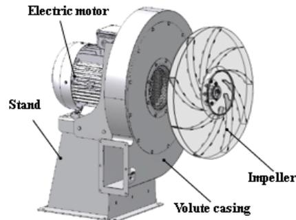
FIGURE 4. Three-dimensional geometry of S-HP 470/35-105/20.
