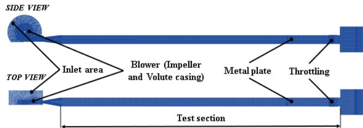
FIGURE 9. Three-dimensional view on a grid for the study of radial high-pressure blowers.
