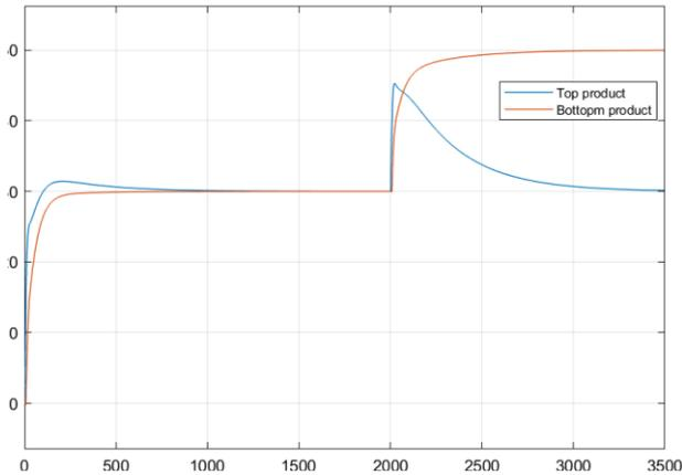
Fig. 13. PI control with change of setpoint on bottom product
