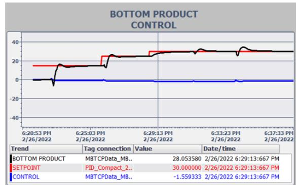
Fig. 28 SCADA - PI real time control of the bottom product
