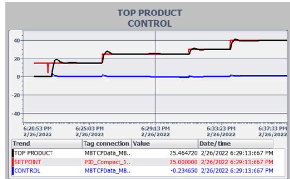
Fig. 27 SCADA - PI real time control of the top product
