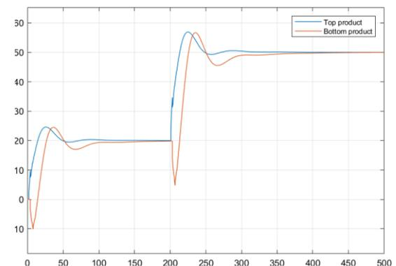
Fig. 6. PI control - change of setpoint
