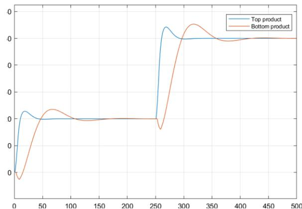
Fig. 18. PI control of discrete model with decoupling matrix - change setpoint
