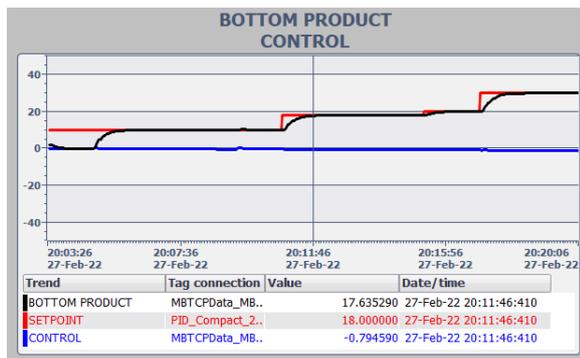
Fig. 31. Bottom Product control with PI and decoupling matrix
