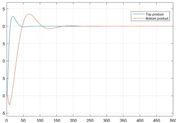
Fig. 17. PI control of discrete model of rectification column with decoupling matrix
