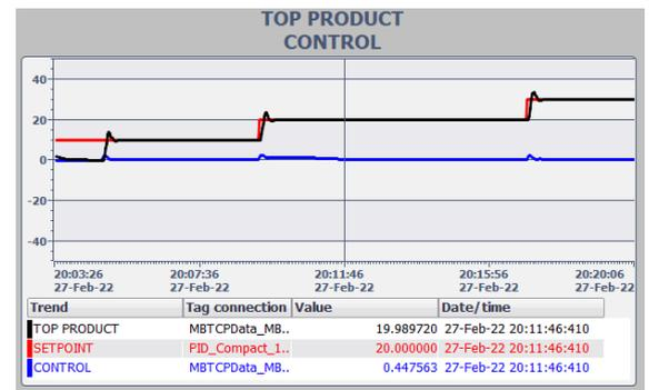
Fig. 30. Top Product control with PI and decoupling matrix
