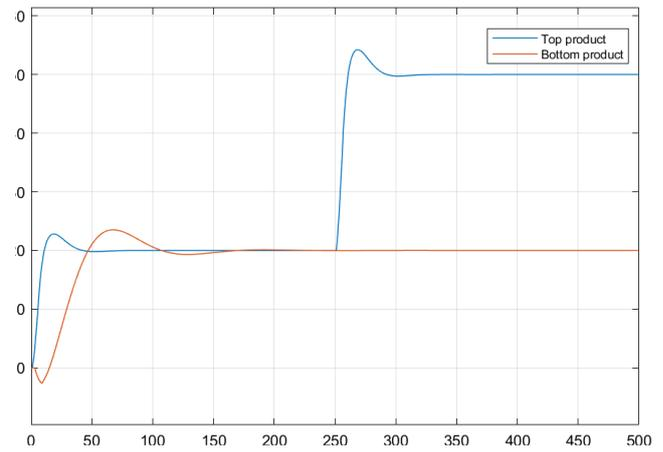
Fig. 19. PI control of discrete model of rectification column with decoupling matrix - change setpoint of top product
