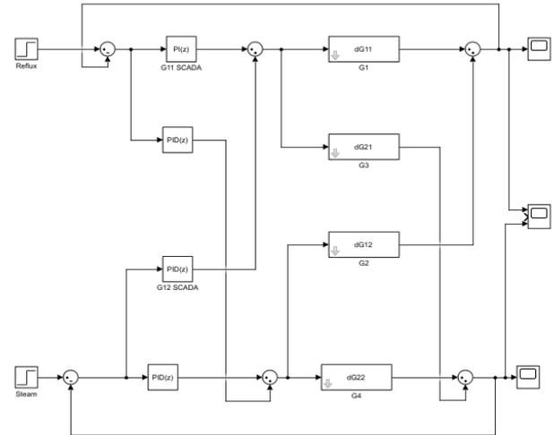
Fig. 9. Simulink scheme of discrete PI control
