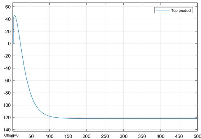
Fig. 7. Step response from discrete model of rectification column
