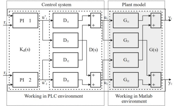
Fig. 14. Structural scheme of multivariable object with decoupling matrix
