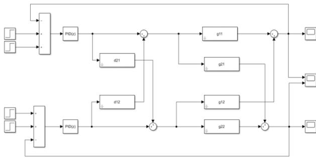
Fig. 16. Simulink scheme of PI control of multivariable model of rectification column with decoupling matrix
