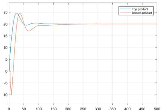
Fig. 5. PI control of continuous model of rectification column
