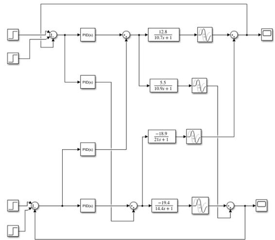
Fig. 4. PI control of continuous model of rectification column
