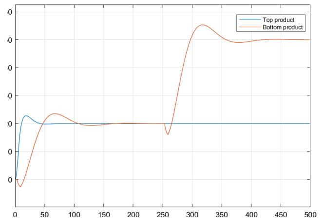
Fig. 20. PI control of discrete model of rectification column with decoupling matrix - change of setpoint of bottom product
