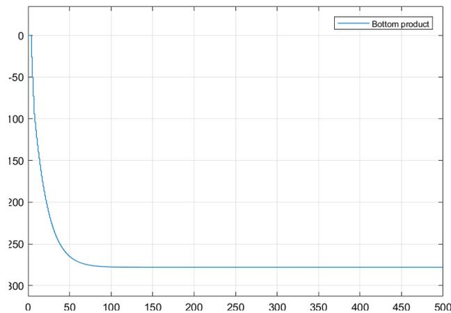
Fig. 8. Step response from bottom product of discrete model of rectification column
