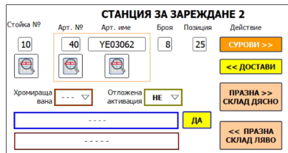
Fig. 8. Loading and unloading dialog system of Load station 2
