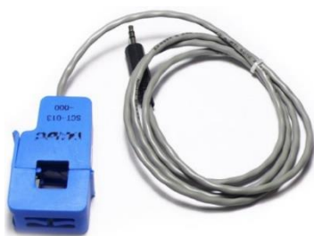
Fig. 5. General view of the current transformer
