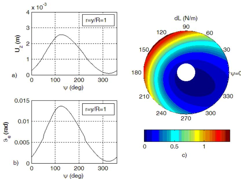
Fig. 7: Third iteration. a) Vertical bending deformation,  $U_z$ , in the blade tip; b) Torsional deformation,  $\theta_e$ , in the blade tip; c) Lift distribution,  $dL$
