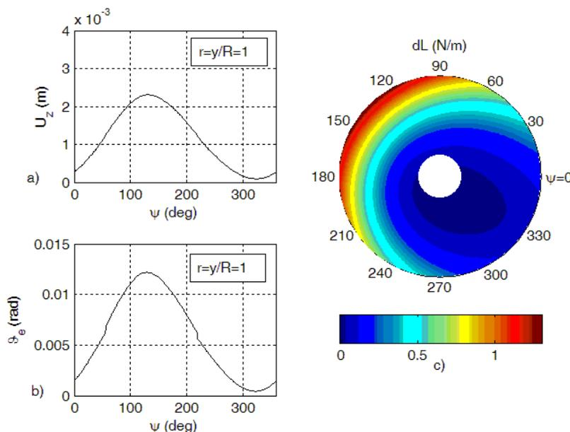
Fig. 5: First iteration. a) Vertical bending deformation,  $U_z$ , in the blade tip; b) Torsional deformation,  $\theta_e$ , in the blade tip; c) Lift distribution,  $dL$
