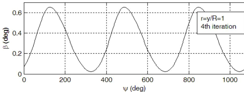
Fig. 9: Azimuthal variation of the coning angle  $\beta$
