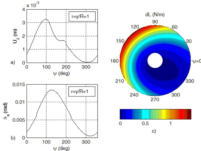
Fig. 6: Second iteration. a) Vertical bending deformation,  $U_z$ , in the blade tip; b) Torsional deformation,  $\theta_e$ , in the blade tip; c) Lift distribution,  $dL$
