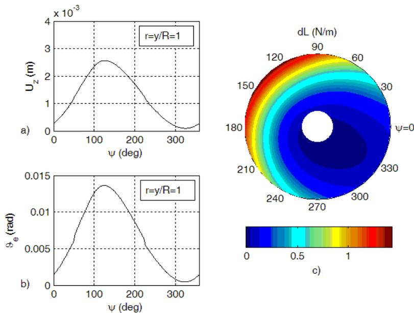
Fig. 8: Forth iteration. a) Vertical bending deformation,  $U_z$ , in the blade tip; b) Torsional deformation,  $\theta_e$ , in the blade tip; c) Lift distribution,  $dL$
