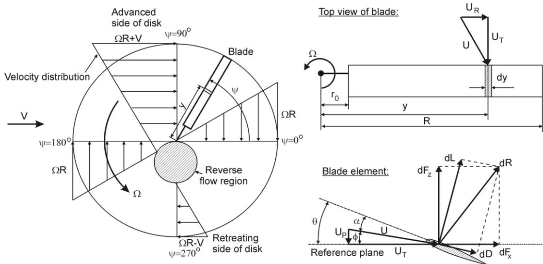
Fig. 2: Incident velocities and aerodynamic forces at a blade element
