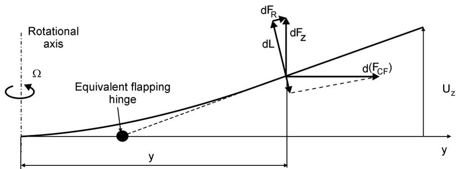
Fig. 3: Equilibrium of blade element aerodynamic and centrifugal forces
