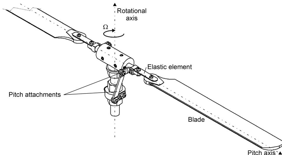
Fig.1: Sketch of a pattern hingeless rotor
