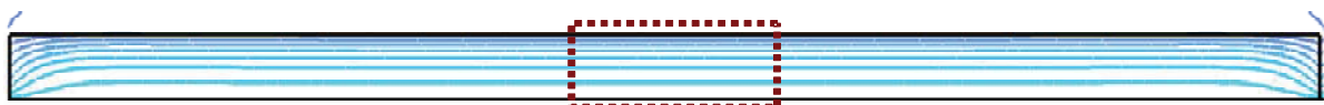
Figure 4. . Temperature distribution in detail's depth obtained for T_{\text{Heater}} 652^{\circ}\text{C} and time 28 s.
