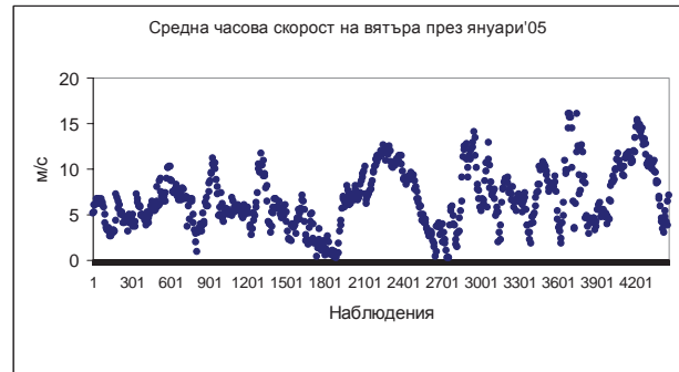
Fig.12. Hourly average 10 min. course of wind speed (m/s) during January'05 near Kavarna, h=50 m.a.g.l.
