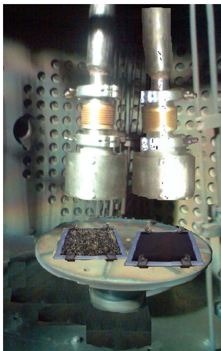
Fig.2. Magnetrons for catalyst sputtering in vacuum
