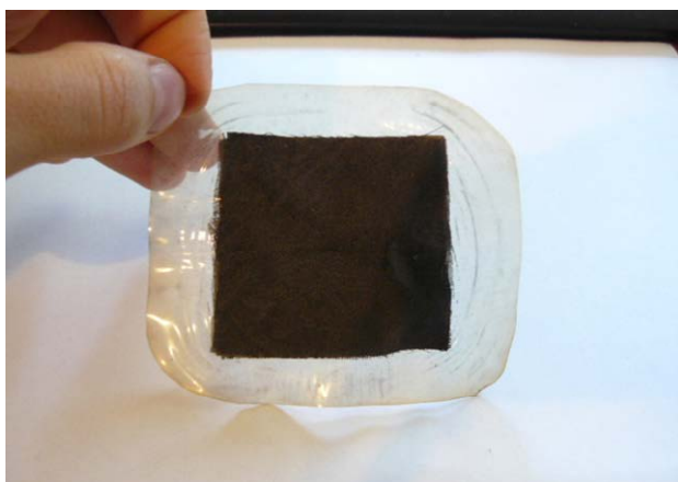
Fig.4. MEA prepared in accordance with the current study
