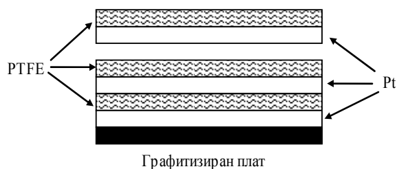
Fig.3. Block diagram of electrode-catalyst structure of MEA
