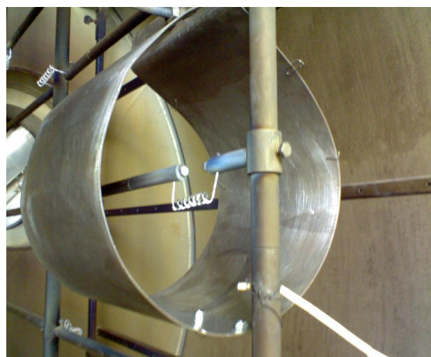
Fig.1. Tungsten evaporator with chromium-nickel sheet iron screen.
