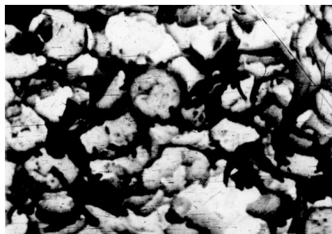
Fig.4.a. Microphoto of structure of filled test bodies – the filler’s particles are isolated in a thermoplastic matrix.
