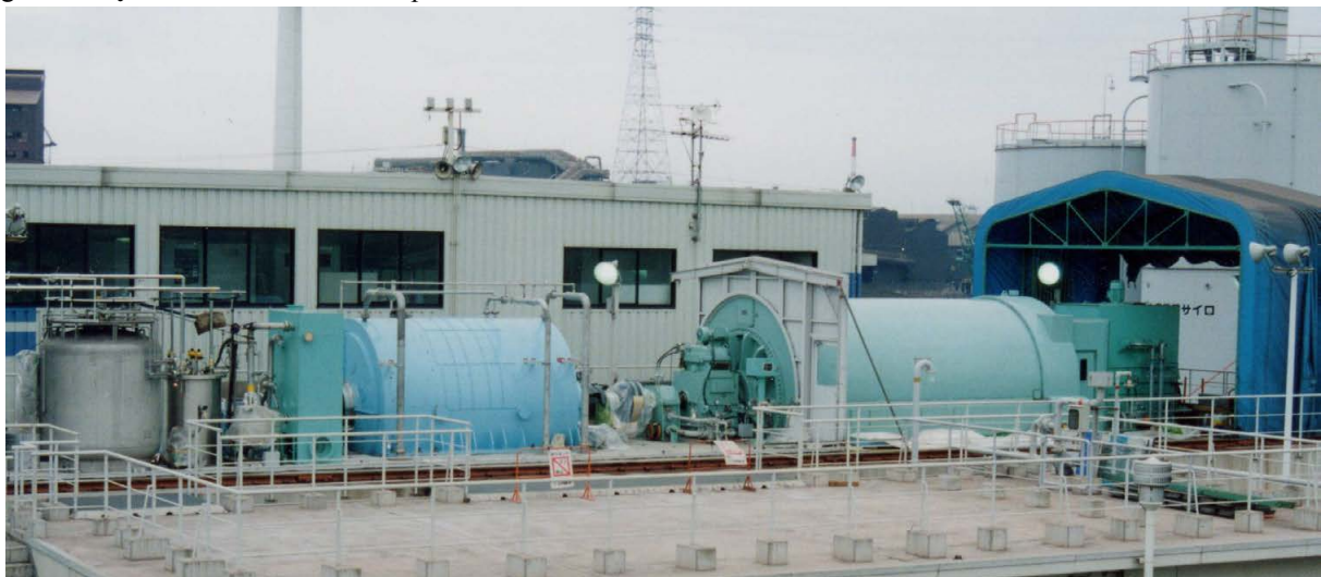
Fig.2. 70MW superconducting generator developed by the Super GM project (Phase I) at the test site. The generator (left side) was driven by a synchronous motor (right side).
