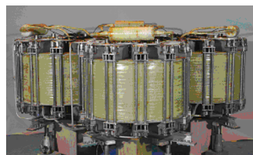
Four Pole 10MJ NbTi Coil Superconducting Model Coil
