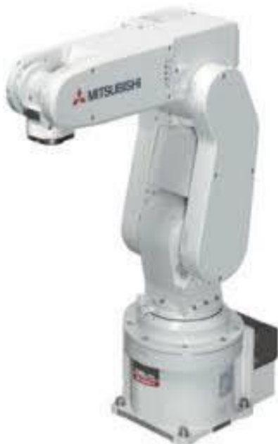
Fig. 1. Robot Mitsubishi Electric RV-2F-Q1-S15 – 6-axis
