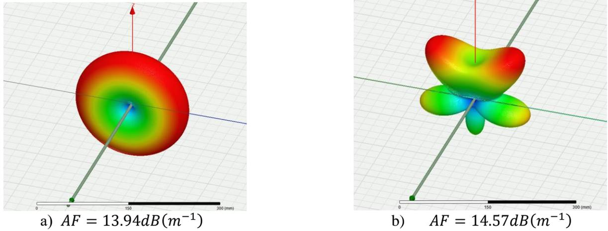
**Fig. 4.** Simulated 3D antenna patterns for resonant half wave reference dipole antenna at 200 MHz, horizontal polarization, height above ground 1.5 m:
