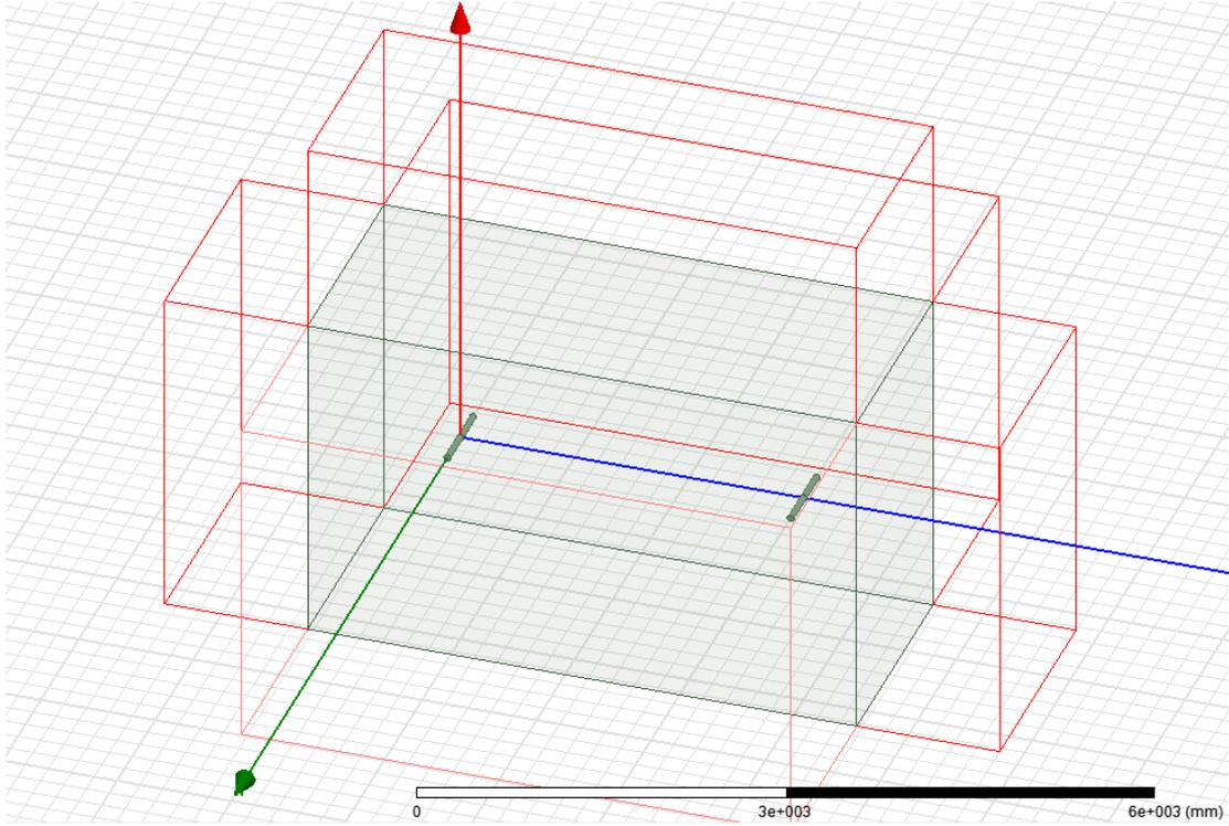
**Fig. 2.** “Ideal” anechoic chamber model used for full electromagnetic simulations
