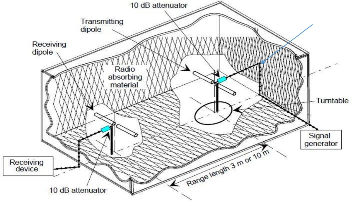
**Fig. 1.** NSA measurement standard test set up according to ETSI102.321 V1.1.1
