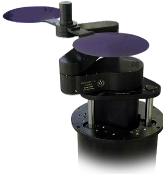
Fig. 6. Hybrid parallel-serial structure of substrate handling robots
